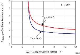
Figure 7. On Resistance vs. Gate Voltage
