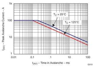
Figure 11. Single Pulse Unclamped Inductive Switching
