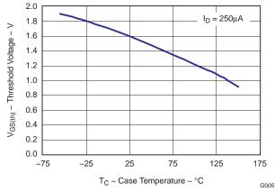
Figure 6. Threshold Voltage vs. Temperature
