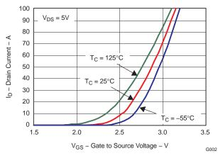
Figure 3. Transfer Characteristics
