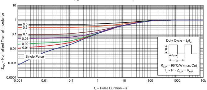
Figure 1. Transient Thermal Impedance
