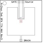
Max  $R_{\theta JA} = 50$ °C/W when mounted on 1inch<sup>2</sup> of 2 oz. Cu.
