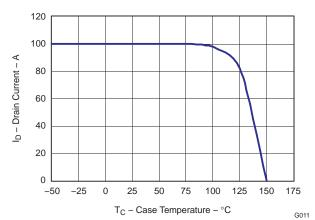
Figure 12. Maximum Drain Current vs. Temperature
