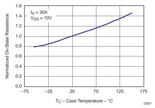
Figure 8. On Resistance vs. Temperature
