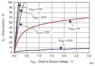
Figure 2. Saturation Characteristics
