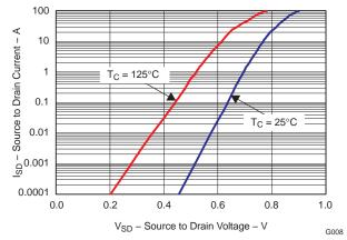
Figure 9. Typical Diode Forward Voltage
