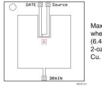
Max  $R_{\theta JA} = 58^{\circ}C/W$ when mounted on 1 in<sup>2</sup> (6.45 cm<sup>2</sup>) of 2-oz (0.071-mm) thick Cu.
