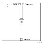
Max  $R_{\theta,JA} = 165^{\circ}C/W$ when mounted on a minimum pad area of 2-oz (0.071-mm) thick) Cu.
