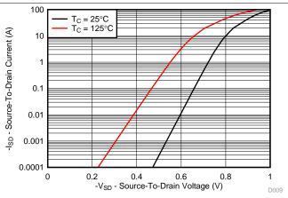
Figure 9. Typical Diode Forward Voltage
