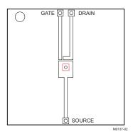
Max  $R_{\theta JA} = 175^{\circ}C/W$  when mounted on minimum pad area of 2 oz. Cu.
