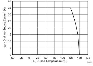
Figure 11. Maximum Drain Current vs Temperature
