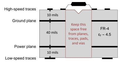
Figure 31. Recommended Layer Stack
