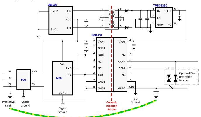
Figure 27. Application Circuit
