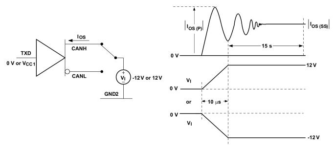
Figure 17. Driver Short-Circuit Current Test Circuit and Waveforms
