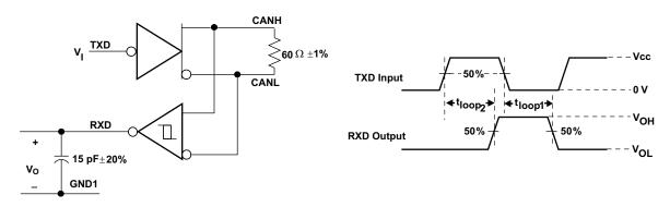
Figure 15. t<sub>LOOP</sub> Test Circuit and Voltage Waveforms
