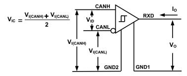
Figure 11. Receiver Voltage and Current Definitions
