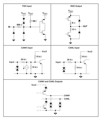
Figure 26. Equivalent I/O Schematics
