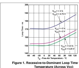
Figure 1. Recessive-to-Dominant Loop Time vs Free-Air Temperature (Across Vcc)
