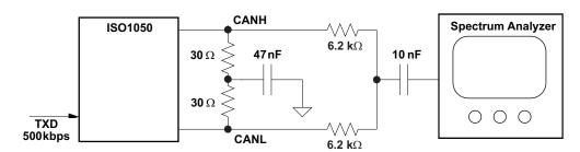
Figure 20. Electromagnetic Emissions Measurement Setup
