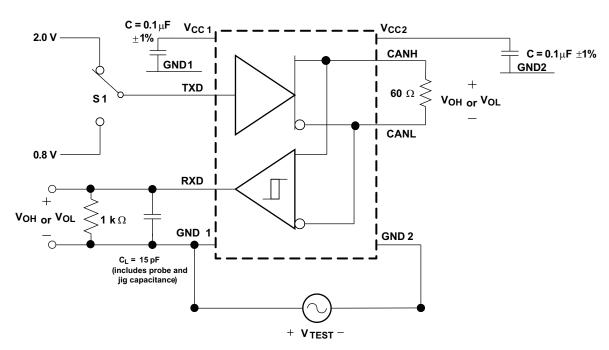
Figure 19. Common-Mode Transient Immunity Test Circuit
