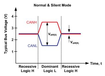
Figure 23. Bus States (Physical Bit Representation)
