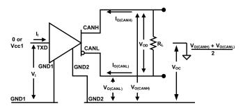
Figure 7. Driver Voltage, Current and Test Definitions
