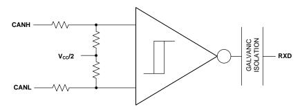
Figure 24. Simplified Recessive Common Mode Bias and Receiver
