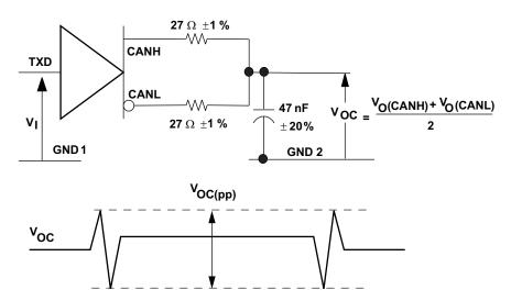
Figure 14. Peak-to-Peak Output Voltage Test Circuit and Waveform
