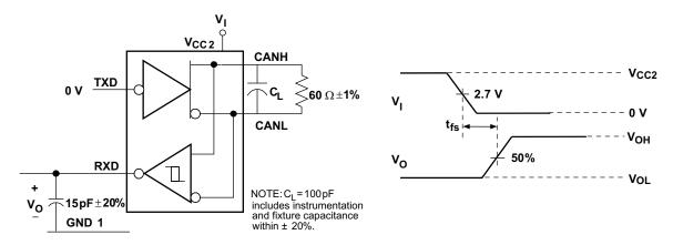
Figure 18. Fail-Safe Delay Time Test Circuit and Voltage Waveforms
