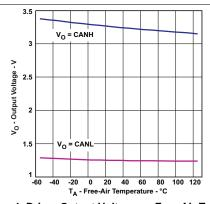
Figure 4. Driver Output Voltage vs Free-Air Temperature
