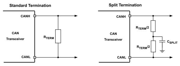
Figure 29. CAN Bus Termination Concepts
