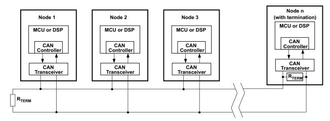
Figure 28. Typical CAN Bus
