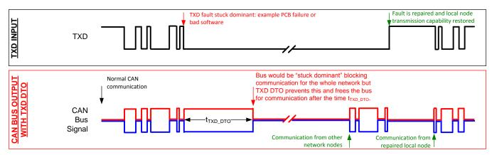
Figure 25. Example Timing Diagram for Devices With TXD DTO
