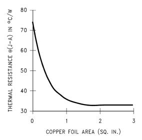
Figure 24. R<sub>0JA</sub> vs. Copper (1 ounce) Area for the DDPAK/TO-263 Package
