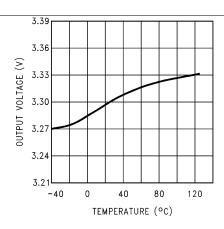
Figure 1. Output Voltage vs Temperature (2.5 V)
