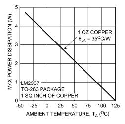
Figure 25. Maximum Power Dissipation vs. T<sub>AMB</sub> for the DDPAK/TO-263 Package
