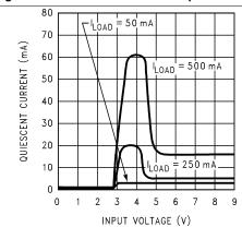
Figure 4. Quiescent Current vs Output Current (3.3 V)
