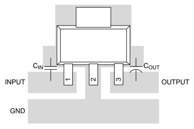
Figure 22. LM2937 SOT-223-4 Layout
