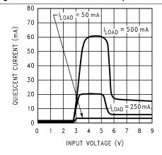
Figure 5. Quiescent Current vs Input Voltage (2.5 V)
