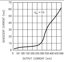
Figure 3. Quiescent Current vs Output Current (2.5 V)
