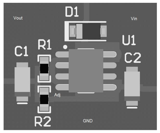
Figure 9. LM337L Layout Example
