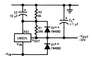
When CL is larger than 20  $\mu$ F, D1 protects the LM337L in case the input supply is shorted. When C2 is larger than 10  $\mu$ F and  $\neg$ VOUT is larger than  $\neg$ 25V, D2 protects the LM337L in case the output is shorted.
