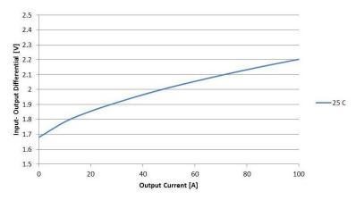
Figure 7. Dropout Voltage across Load Current at 25°C (△Vout < 100 mV
