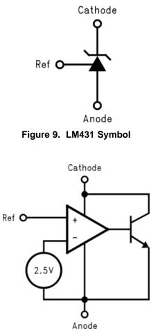
Figure 10. LM431 Block Diagram
