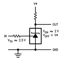
Figure 16. Single Supply Comparator With Temperature Compensated Threshold
