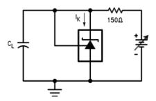
Figure 4. Test Circuit for Curve A Above
