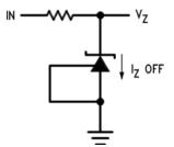
Figure 8. Test Circuit for OFF-State Current
