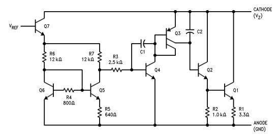
Figure 11. Equivalent Circuit
