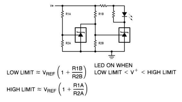
Figure 22. Voltage Monitor
