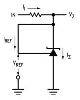
Figure 6. Test Circuit for  $V_Z = V_{REF}$
