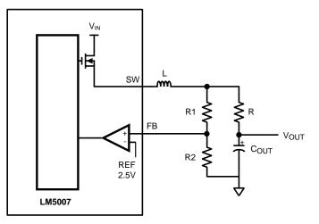
Figure 4. Low Ripple Output Configuration
