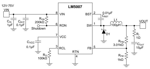
Figure 7. 12-V to 75-V Input and 10-V, 400-mA Output Buck Converter
