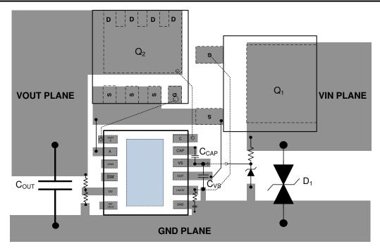
Figure 12-2. PCB Layout Example for Common Source Configuration
