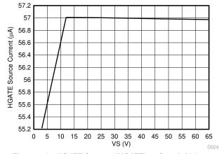
Figure 7-14. HGATE Current (IHGATE) vs Supply Voltage
