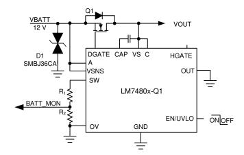
Figure 9-2. Configuring LM7480x-Q1 for Ideal Diode Only
