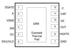
Figure 6-1. WSON 12-Pin DRR Transparent Top View
