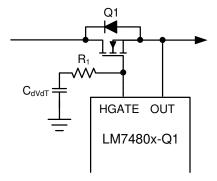
Figure 9-3. Inrush Current Limiting
