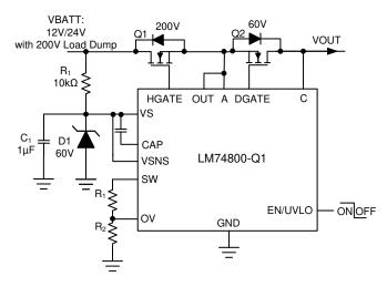
Figure 9-6. Ideal Diode with 200-V Unsupressed Load Dump Protection
