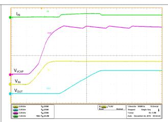
Figure 10-8. Startup 12 V showing Charge Pump VCAP
