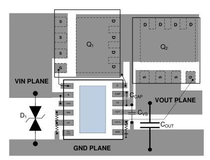
Figure 12-1. PCB Layout Example for Common Drain Configuration
