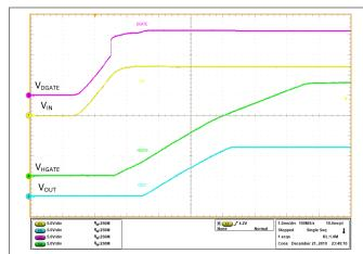
Figure 10-7. Startup 12 V with EN Pulled to VIN
