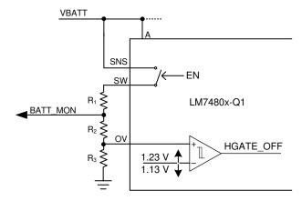
Figure 9-4. Programming Overvoltage Threshold and Battery Sensing
