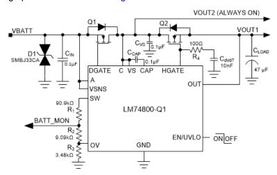
Figure 10-1. Typical Application Circuit - 12-V Reverse Battery Protection and Overvoltage Protection
