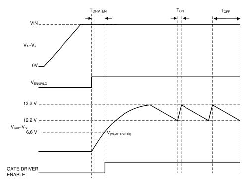
Figure 9-1. Charge Pump Operation
