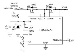
Ideal Diode with 200-V Load Dump Protection
