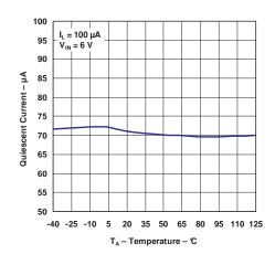
Figure 10. Quiescent Current vs Temperature ( $I_L = 100 \mu A$ )
