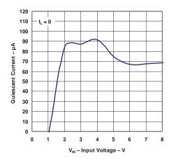
Figure 6. Quiescent Current vs Input Voltage (I<sub>L</sub> = 0)
