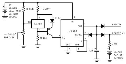
For values shown, regulator shuts down when  $V_{in}$  < 5.5 V and turns on again at 6 V. Current drain in disconnected mode is approximately 150  $\mu$ A.
