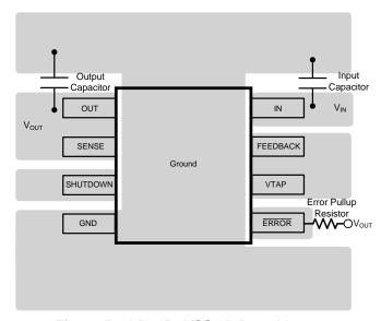
Figure 57. LP2951 VSSOP Board Layout
