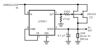
Figure 44. 300-mA Regulator with 0.75-V Dropout
