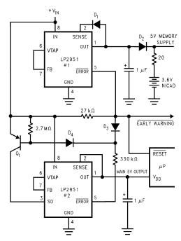
Figure 48. Regulator With Early Warning and Auxiliary Output
