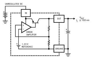
Figure 33. LP2950-N Functional Block Diagram
