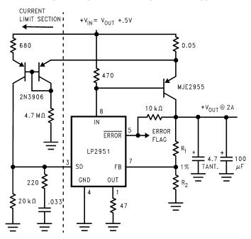
Figure 50. 2-A Low Dropout Regulator
