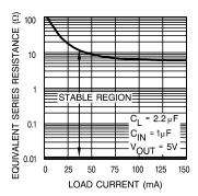
Figure 37. Output Capacitor ESR Range
