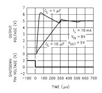
Figure 38. LP2951-N Enable Transient
