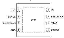
Connect DAP to GND at device pin 4.
