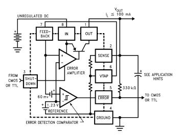
Figure 34. LP2951-N Functional Block Diagram
