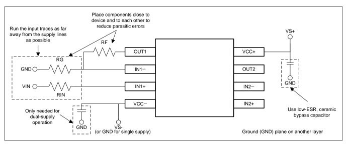
Figure 9. Operational Amplifier Board Layout for Noninverting Configuration
