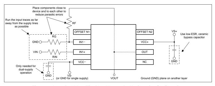
Figure 8. Operational Amplifier Board Layout for Noninverting Configuration
