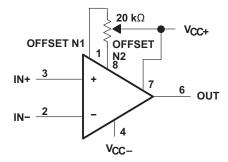
Figure 2. Input Offset-Voltage Null Circuit
