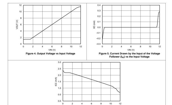
VIN (V) Figure 6. Current Drawn from Supply (I<sub>CC</sub>) vs the Input Voltage
