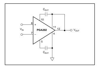
FIGURE 5. Output Filtering.
