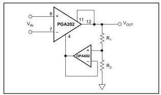
FIGURE 3. Gain Increase with Buffered Attenuator.
