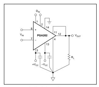
FIGURE 1. Basic Circuit Connections.
