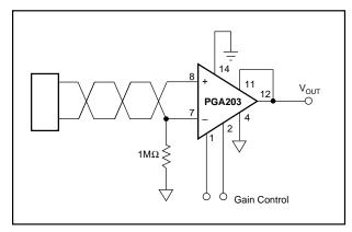
FIGURE 9. Floating Source Programmable Gain Instrumentation Amplifier.
