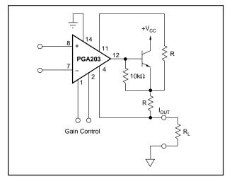
FIGURE 12. Programmable Current Source.
