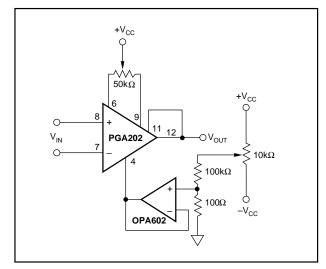
FIGURE 2. Offset Adjustment Circuits.
