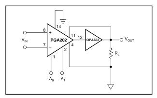
FIGURE 4. Current Boosting the Output.
