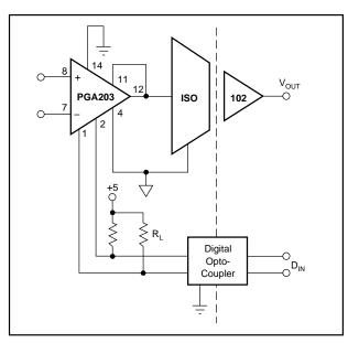
FIGURE 6. Isolated Programmable Gain Instrumentation Amplifier.
