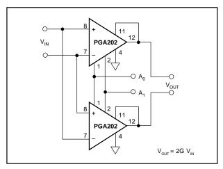
FIGURE 11. Programmable Differential In/Differential Out Amplifier.
