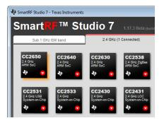
After installing the tool, connect the EB to the PC using the USB cable and start SmartRF Studio. Select the "2.4 GHz" tab and click the refresh ("Find device") button in the lower right corner. Studio will now find the connected SmartRF06EB. Double click on the detected SmartRF06EB to launch the CC2650 device control panel.
