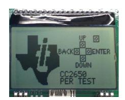
Turn on power with the Main Power switch. You Then select the protocol. should now see the Texas Instruments logo and a short description of the buttons on the LCD. Pushing any of the five buttons on the board will take you to the main menu.
