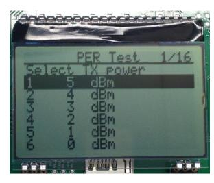
On the transmitter, select the desired output power.
