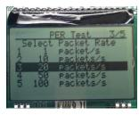
Then select the packet rate (number of packets to transmit per second).
