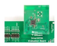
CC2650EM Insert а board into the SmartRF06EB as shown above.
