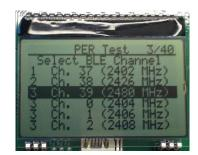
Then select the type of test you want to run. Packet mode is the Packet Error Rate test. CW is a continuous wave signal, either modulated or unmodulated.
