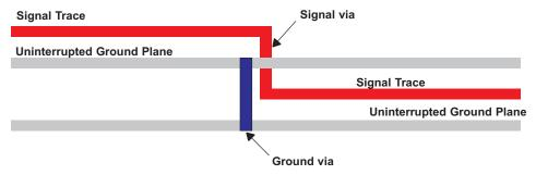
Figure 22. Ground Via Location (Side View)
