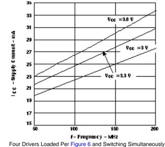
Figure 1. SN55LVDS31, SN65LVDS31 Supply Current vs Frequency
