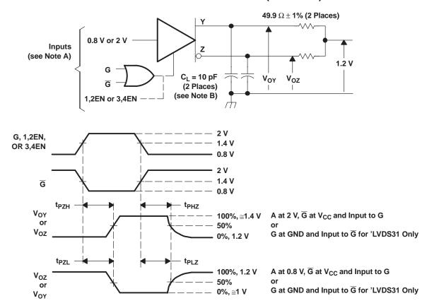
NOTES: A. All input pulses are supplied by a generator having the following characteristics:  $t_r$  or  $t_f < 1$  ns, pulse repetition rate (PRR) = 0.5 Mpps, pulse width =  $500 \pm 10$  ns.
