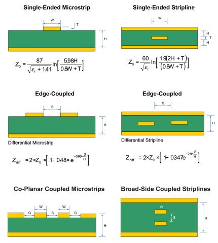
Figure 12. Controlled-Impedance Transmission Lines
