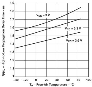
Figure 3. High-to-Low Propagation Delay Time vs Free-Air Temperature
