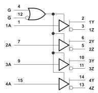
SN65LVDS3487 logic diagram (positive logic)
