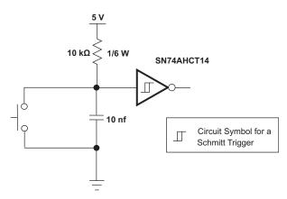
Figure 3. Switch De-bouncer Using Schmitt Trigger Inverter
