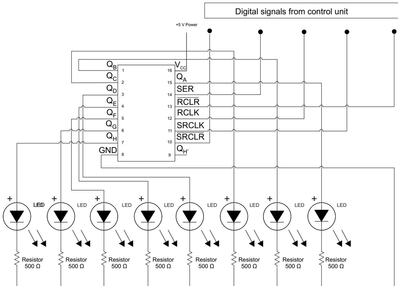
**Figure 3. Application Schematic**
