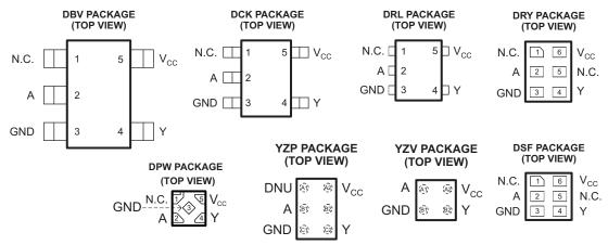
N.C. – No internal connection See mechanical drawings for dimensions. DNU – Do not use
