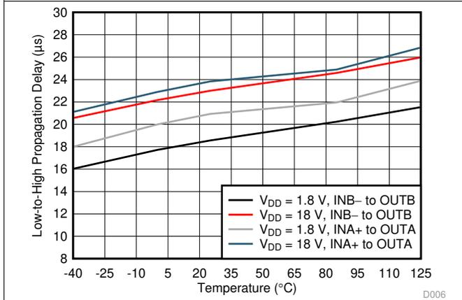
Figure 6. Propagation Delay vs Temperature (Low-to-High Transition at the Inputs)
