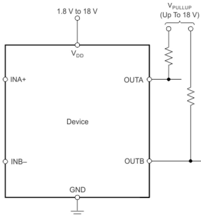
Figure 16. Interfacing to Voltages Other Than  $V_{DD}$
