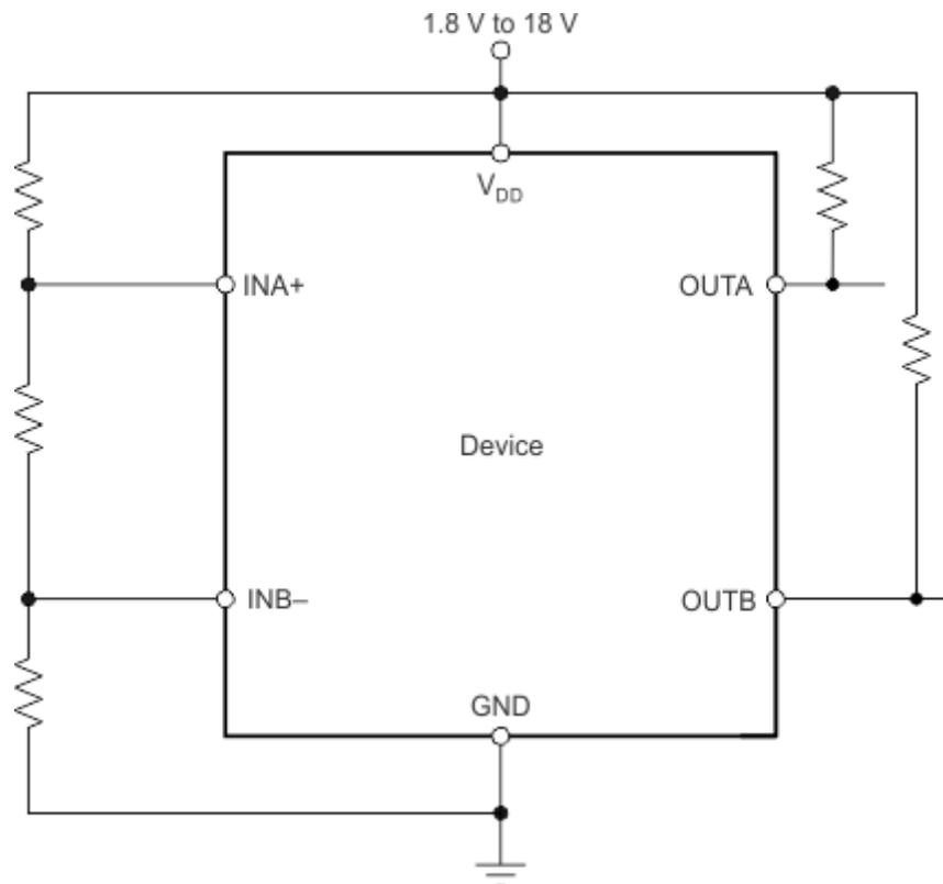
Figure 17. Monitoring the Same Voltage as  $V_{DD}$
