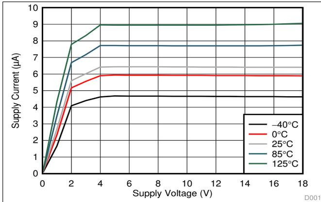
Figure 2. Supply Current ( $I_{DD}$ ) vs Supply Voltage ( $V_{DD}$ )
