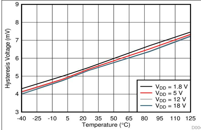
Figure 4. Hysteresis ( $V_{hys}$ ) vs Temperature
