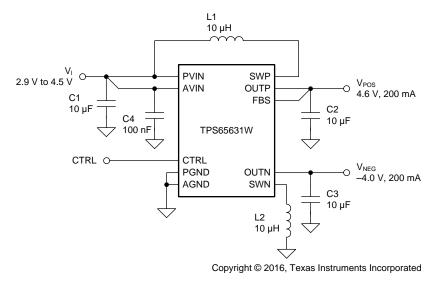
Figure 8. Typical Application Schematic
