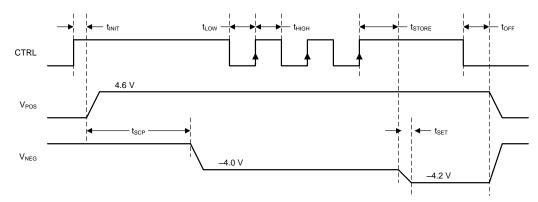
Figure 7. Programming  $V_{NEG}$  Using the CTRL Pin
