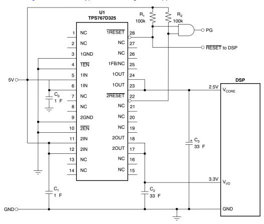
Figure 25. Dual-Voltage DSP Application
