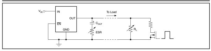
Figure 20. Test Circuit for Typical Regions of Stability (Figure 21 through Figure 24) (Fixed Output Options)
