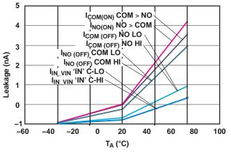
Figure 4. Leakage Current vs Temperature ( $V_{+} = 5.5 V$ )
