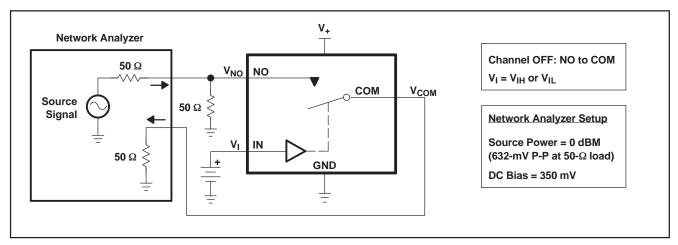
Figure 19. OFF Isolation (O<sub>ISO</sub>)
