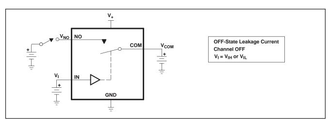
Figure 14. OFF-State Leakage Current (I<sub>COM(OFF)</sub>, I<sub>NO(OFF)</sub>)
