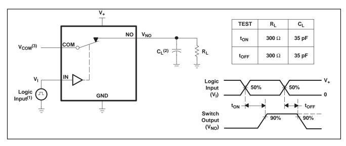
(1) All input pulses are supplied by generators having the following characteristics: PRR  $\leq$  10 MHz, Z<sub>O</sub> = 50  $\Omega$ , t<sub>f</sub> < 5 ns, t<sub>f</sub> < 5 ns.
