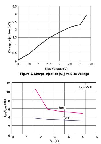
Figure 6.  $t_{\text{ON}}$  and  $t_{\text{OFF}}$  vs Supply Voltage
