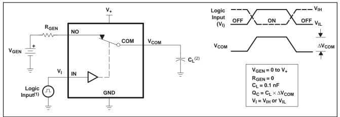
(1) All input pulses are supplied by generators having the following characteristics: PRR  $\leq$  10 MHz, Z<sub>O</sub> = 50  $\Omega$ , t<sub>r</sub> < 5 ns, t<sub>f</sub> < 5 ns.
