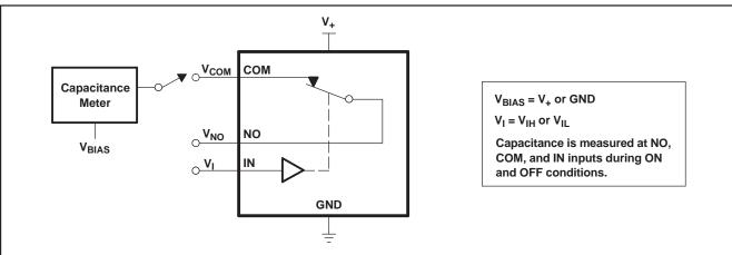
Figure 16. Capacitance (C<sub>I</sub>, C<sub>COM(OFF)</sub>, C<sub>COM(ON)</sub>, C<sub>NO(OFF)</sub>, C<sub>NO(ON)</sub>)
