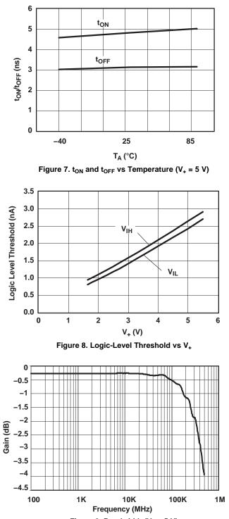
Figure 9. Bandwidth (V<sub>+</sub> = 5 V)
