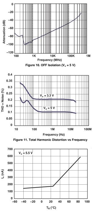
Figure 12. Power-Supply Current vs Temperature (V<sub>+</sub> = 5 V)
