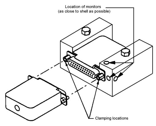
Figure 4 Vibration and Physical Shock Mounting and Clamping Locations
