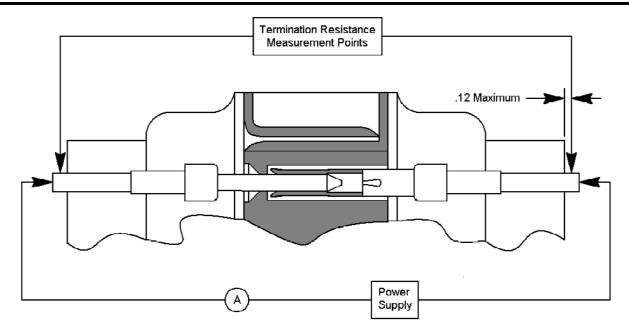
Figure 3 Termination Resistance Measurement Points
