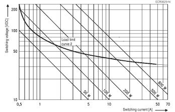
Load limit curve: safe shutdown, no stationary arc/make contact. Load limit curve measured with low inductive resistors verified for 1000 switching events
