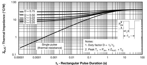
Fig. 4 - Maximum Thermal Impedance Z<sub>thJC</sub> Characteristics (Per Leg)
