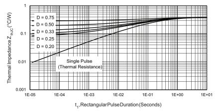
Fig. 4 - Maximum Thermal Impedance  $Z_{thJC} \mbox{ Characteristics}$
