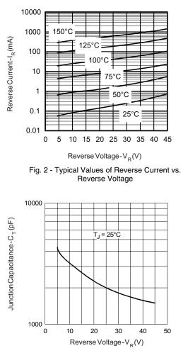
Fig. 3 - Typical Junction Capacitance vs. Reverse Voltage
