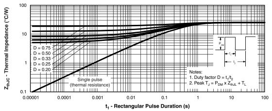
Fig. 4 - Maximum Thermal Impedance  $Z_{thJL}$  Characteristics
