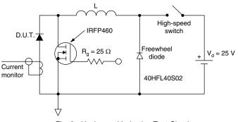
Fig. 8 - Unclamped Inductive Test Circuit
