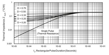
Fig. 4 - Maximum Thermal Impedance Z<sub>thJC</sub> Characteristics
