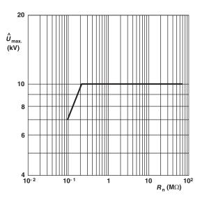
Maximum allowed peak pulse voltage in accordance with IEC 60065, 14.1.a); 50 discharges from a 1 nF capacitor charged to  $\hat{U}_{\text{max}}$ ; 12 discharges/min (drift  $\Delta R/R \leq 2 \%$ )
