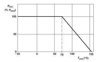
Maximum dissipation ( $P_{\rm max}$ ) in percentage of rated power as a function of the ambient temperature ( $T_{\rm amb}$ )
