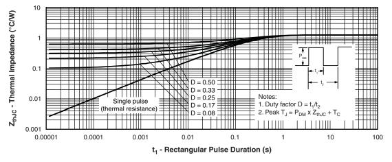
Fig. 4 - Maximum Thermal Impedance Z<sub>thJC</sub> Characteristics (Per Leg)
