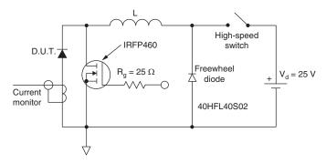
Fig. 8 - Unclamped Inductive Test Circuit
