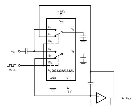
Figure 8. Band-Pass Switched Capacitor Filter
