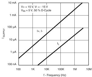
**Power Supply Currents vs. Switching Frequency**
