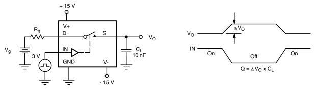
Figure 7. Charge Injection
