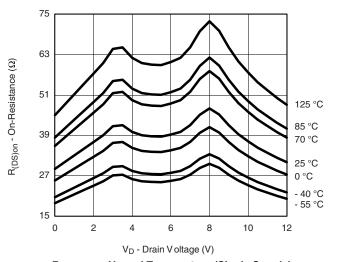
R<sub>DS(on)</sub> vs. V<sub>D</sub> and Temperature (Single Supply)
