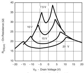
R<sub>DS(on)</sub> vs. V<sub>D</sub> (Dual Supply)
