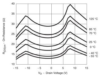
R<sub>DS(on)</sub> vs. V<sub>D</sub> and Temperature (Dual Supply)
