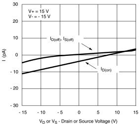
Leakage Currents vs. Analog Voltage
