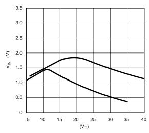
Input Switching Threshold vs. Supply Voltages
