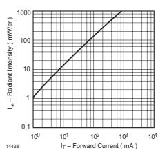
Figure 6. Radiant Intensity vs. Forward Current
