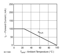
Figure 2. Forward Current vs. Ambient Temperature
