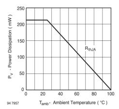
Figure 1. Power Dissipation vs. Ambient Temperature
