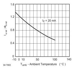
Figure 8. Rel. Radiant Intensity/Power vs. Ambient Temperature
