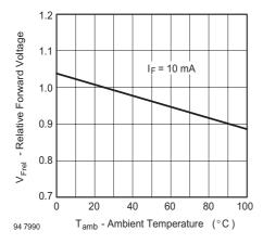
Figure 5. Relative Forward Voltage vs. Ambient Temperature
