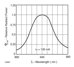
Figure 9. Relative Radiant Power vs. Wavelength
