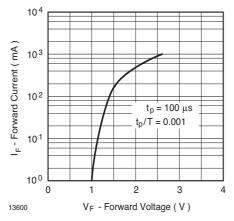
Figure 4. Forward Current vs. Forward Voltage
