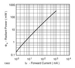
Figure 7. Radiant Power vs. Forward Current
