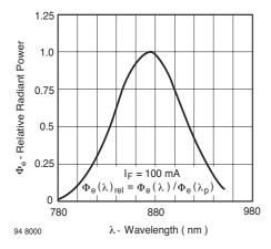
Figure 9. Relative Radiant Power vs. Wavelength
