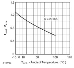
Figure 8. Rel. Radiant Intensity/Power vs. Ambient Temperature
