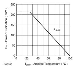
Figure 1. Power Dissipation vs. Ambient Temperature
