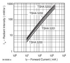
Figure 6. Radiant Intensity vs. Forward Current
