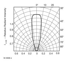
Figure 10. Relative Radiant Intensity vs. Angular Displacement
