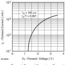
Figure 4. Forward Current vs. Forward Voltage
