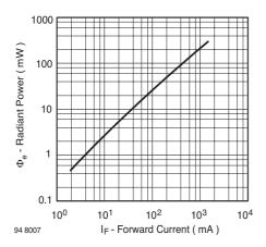
Figure 7. Radiant Power vs. Forward Current
