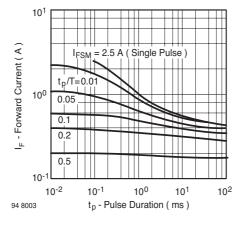
Figure 3. Pulse Forward Current vs. Pulse Duration
