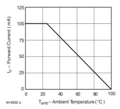
Figure 2. Forward Current vs. Ambient Temperature
