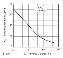
Figure 5. Diode Capacitance vs. Reverse Voltage
