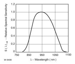
Figure 6. Relative Spectral Sensitivity vs. Wavelength
