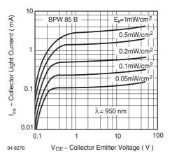
Figure 6. Collector Light Current vs. Collector Emitter Voltage
