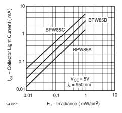
Figure 4. Collector Light Current vs. Irradiance
