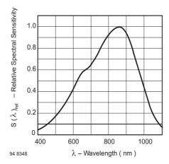
Figure 10. Relative Spectral Sensitivity vs. Wavelength
