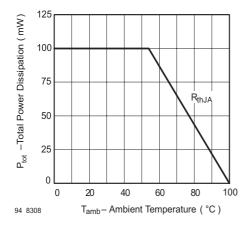
Figure 1. Total Power Dissipation vs. Ambient Temperature
