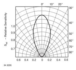
Figure 11. Relative Radiant Sensitivity vs. Angular Displacement
