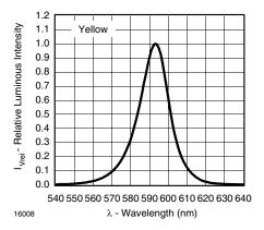
Figure 3. Relative Intensity vs. Wavelength
