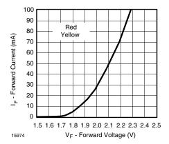
Figure 4. Forward Current vs. Forward Voltage
