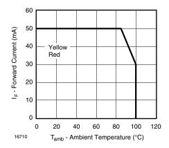
Figure 1. Forward Current vs. Ambient Temperature
