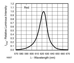
Figure 2. Relative Intensity vs. Wavelength
