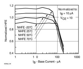
Figure 9. Normalized HFE vs. Base Current and Temp.
