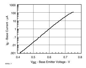
Figure 11. Base Emitter Voltage vs. Base Current
