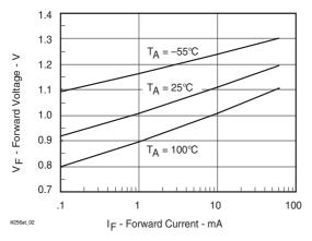
Figure 2. Forward Voltage vs. Forward Current
