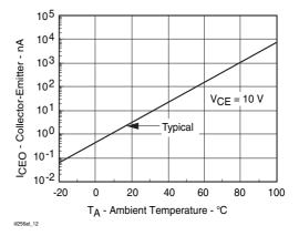
Figure 12. Collector-Emitter Leakage Current vs.Temp.
