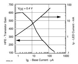
Figure 8. Base Current vs.  $I_F$  and HFE
