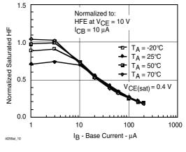
Figure 10. Normalized Saturated HFE vs. Base Current
