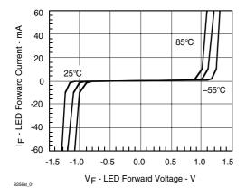
Figure 1. LED Forward Current vs.Forward Voltage
