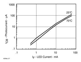
Figure 7. Photocurrent vs. LED Current
