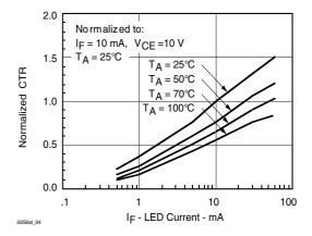
Figure 4. Normalized CTR vs. I<sub>F</sub> and T<sub>amb</sub>
