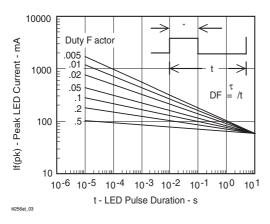
Figure 3. Peak LED Current vs. Duty Factor, Tau
