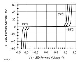
Figure 1. LED Forward Current vs.Forward Voltage
