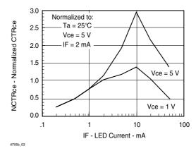
Figure 3. Normalized Non-saturated and Saturated  ${\rm CTR}_{\rm CE}$  vs. LED Current
