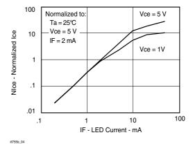
Figure 4. Normalized Non-Saturated and Saturated  $I_{\mbox{\footnotesize{CE}}}$  vs. LED Current
