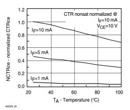
Figure 4. Current Transfer Ratio (normalized) vs. Ambient Temperature
