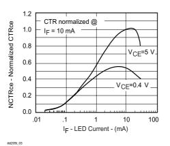
Figure 3. Normalized  $\text{CTR}_{\text{ce}}$  vs. Forward Current
