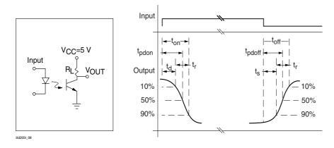
Figure 8. Switching Test Circuit
