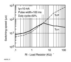
Figure 5. Switching Speed vs. Load Resistor
