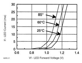
Figure 1. Forward Current vs. Forward Voltage
