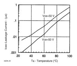
Figure 6. Collector Current vs. Ambient Temperature
