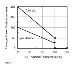
Figure 7. Power Dissipation vs. Ambient Temperature
