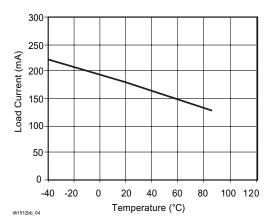
Figure 5. Form B\_Typical Load Current vs. Temperature
