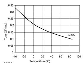
Figure 9. Form A\_Typical Turn-Off vs. Temperature
