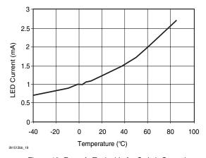
Figure 19. Form A\_Typical  $I_F$  for Switch Operation vs. Temperature
