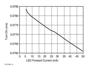
Figure 16. Form B\_Typical Turn-On vs. LED Forward Current
