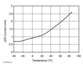
Figure 20. Form A\_Typical I<sub>F</sub> for Switch Dropout vs. Temperature
