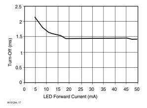
Figure 17. Form B\_Typical Turn-Off vs. LED Forward Current
