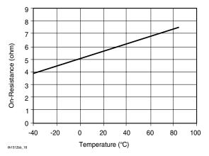
Figure 18. Form B\_Typical On-Resistance vs. Temperature
