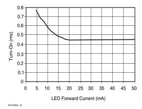
Figure 13. Form A\_Typical Turn-On vs. LED Forward Current
