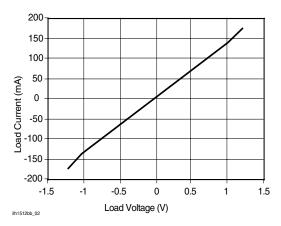
Figure 3. Form A\_Typical Load Current vs. Load Voltage
