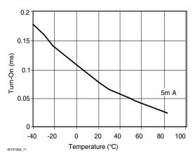
Figure 11. Form B\_Typical Turn-On vs. Temperature
