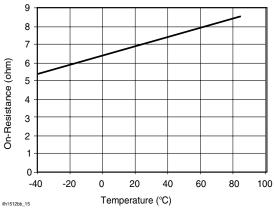
Figure 15. Form A\_Typical On-Resistance vs. Temperature
