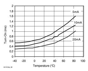
Figure 8. Form A\_Typical Turn-On vs. Temperature
