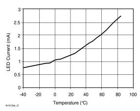
Figure 21. Form B\_Typical  $I_F$  for Switch Operation vs. Temperature
