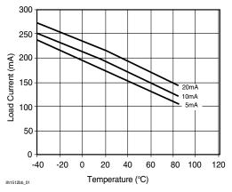
Figure 2. Form A\_Typical Load Current vs. Temperature
