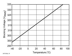
Figure 10. Form B\_Typical Blocking Voltage vs. Temperature
