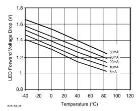
Figure 6. Typical LED Forward Voltage Drop vs. Temperature
