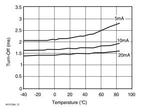
Figure 12. Form B\_Typical Turn-Off vs. Temperature
