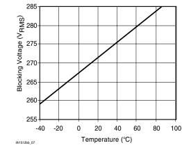
Figure 7. Form A\_Typical Blocking Voltage vs. Temperature
