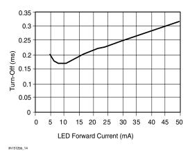
Figure 14. Form A\_Typical Turn-Off vs. LED Forward Current
