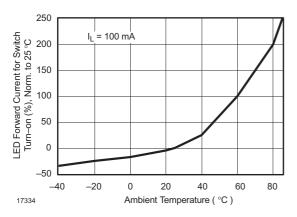
Figure 3. LED Current for Switch Turn-on vs. Temperature
