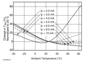
Figure 7. Turn-on Time vs. Temperature
