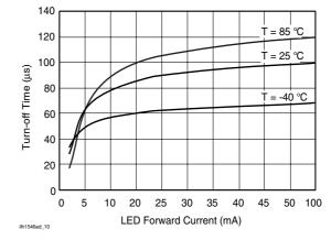
Figure 10. Turn-off Time vs. LED Current
