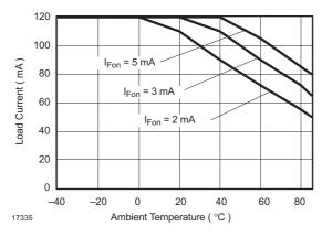
Figure 1. Recommended Operating Conditions
