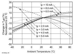
Figure 8. Turn-off Time vs. Temperature
