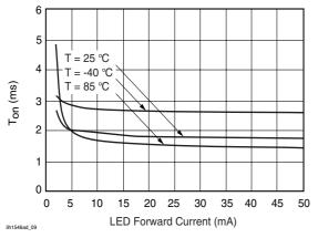
Figure 9. Turn-on Time vs. LED Current
