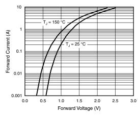
Figure 1. Forward Current vs. Forward Voltage
