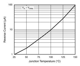
Figure 3. Reverse Current vs. Junction Temperature
