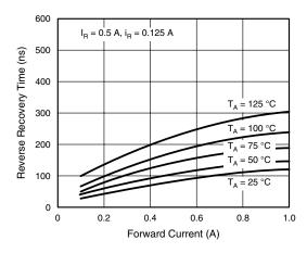
Figure 6. Reverse Recovery Time vs. Forward Current
