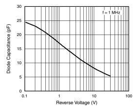
Figure 5. Diode Capacitance vs. Reverse Voltage
