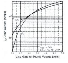
Fig. 3 - Typical Transfer Characteristics
