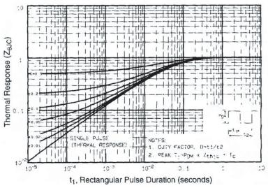
Fig. 11 - Maximum Effective Transient Thermal Impedance, Junction-to-Case
