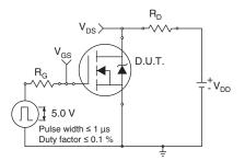
Fig. 10a - Switching Time Test Circuit
