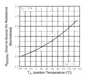
Fig. 4 - Normalized On-Resistance vs. Temperature
