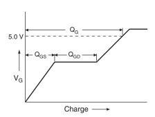
Fig. 13a - Basic Gate Charge Waveform
