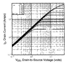
Fig. 2 - Typical Output Characteristics,  $T_C = 150 \, ^{\circ}C$
