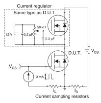
Fig. 13b - Gate Charge Test Circuit
