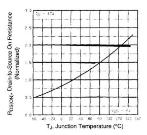
Fig. 4 - Normalized On-Resistance vs. Temperature
