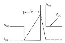
Fig. 12b - Unclamped Inductive Waveforms
