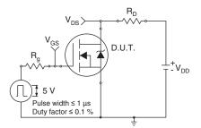
Fig. 10a - Switching Time Test Circuit
