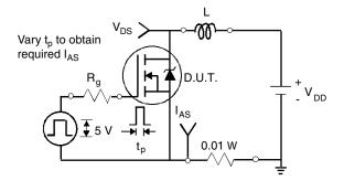
Fig. 12a - Unclamped Inductive Test Circuit
