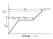
Fig. 13a - Basic Gate Charge Waveform
