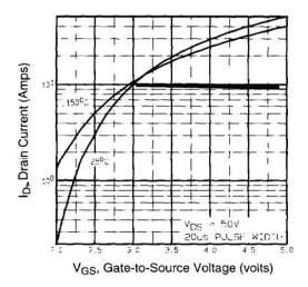
Fig. 3 - Typical Transfer Characteristics
