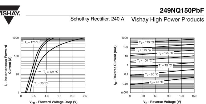
Fig. 1 - Maximum Forward Voltage Drop Characteristics
