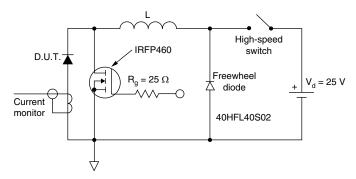
Fig. 8 - Unclamped Inductive Test Circuit
