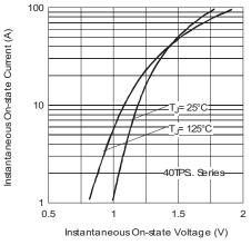
Fig. 7 - On-State Voltage Drop Characteristics
