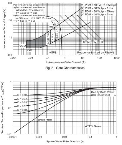
Fig. 9 - Thermal Impedance Z<sub>thJC</sub> Characteristics
