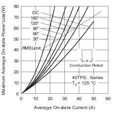
Fig. 4 - On-State Power Loss Characteristics
