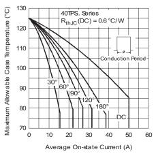
Fig. 2 - Current Rating Characteristics
