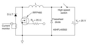
Fig. 8 - Unclamped Inductive Test Circuit
