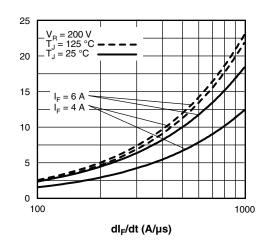
Fig. 6 - Typical Recovery Current vs. dl<sub>F</sub>/dt
